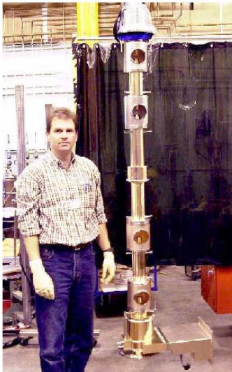
Figure 1. CPI 550 kW klystron during assembly
