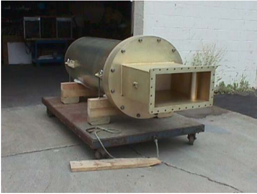
Figure 3. 2.5 MW, 402.5 MHz Glycol/Water RF Load
