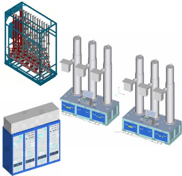
Figure 2. Transmitter components for the superconducting RF systems include the water manifold (upper left), the 3-klystron oil tanks (center and right), and the control racks (lower left).
