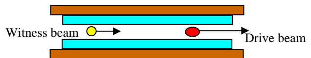
Figure 2: Collinear wakefield experiment setup. Where a high charge beam passing through a dielectric structure will generate high gradient and thus accelerator a trailing witness beam. The drive beam can be either a single or multiple bunches.
