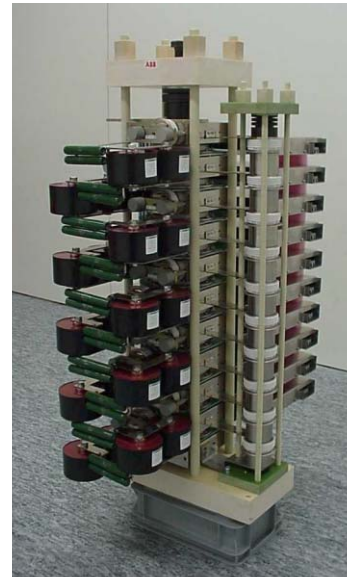
Figure 6: 5SHB 35L45-10-CC Reverse Blocking IGCT Switch with RCD and Press Pack MOV protection.
