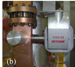
Figure 5: The Photograph of the PV-3040N klystron. (a) Overview of the PV-3040N klystron. (b) Close-up around the klystron ion pump.
