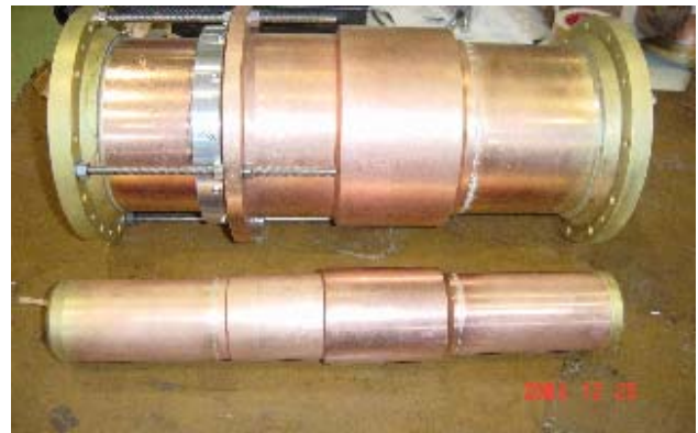
Figure 1: Variable-length WX-203D coaxial waveguide. The outer (upper) and the inner (lower) conductors.
