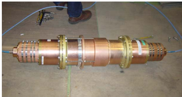
Figure 3: Setup for rf characteristics measurement of a variable-length WX-203D coaxial waveguide.
