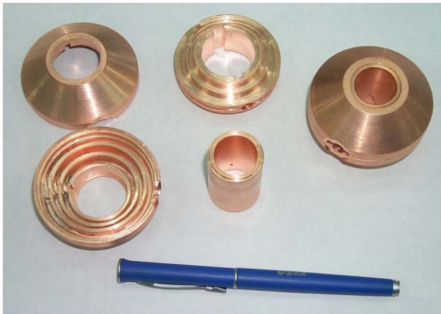
Fig.4 A Prototype Drift-tube assembly and its four parts.
