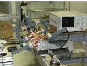
Fig.4. The plunger set-up for nodal measurements.
