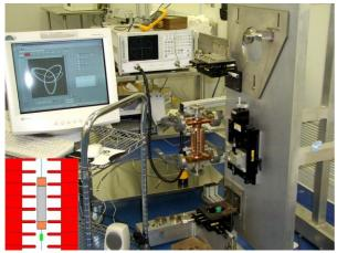
Fig.5. The general arrangement of the bead-pull set-up.
