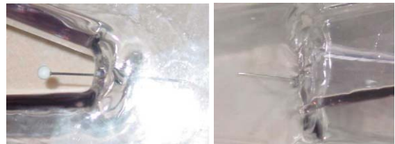
Figure 9: Demonstration of the burned through hole with the 0.8-mm pin.
