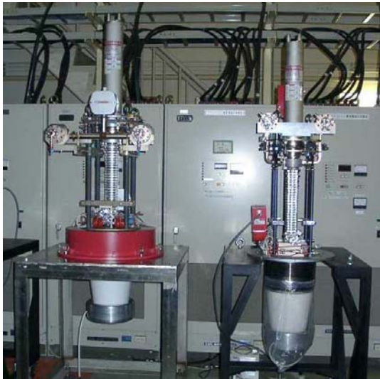
Figure 2: Photo of KEK PPM klystrons, 50MW PPM-1 (right) and 75MW PPM-2 (left).
