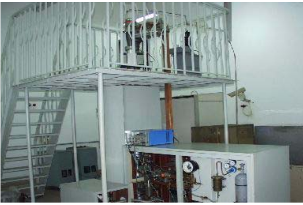
Figure 12: A 4-12MeV electron linac for radiating the power thyristor device.
