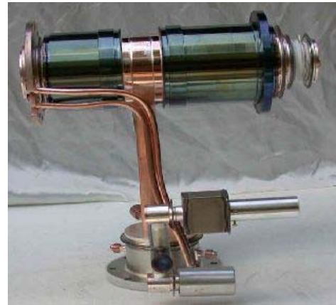
Figure 1: A 6MeV accelerating tube produced by Tsinghua University in cooperation with BVERI.
