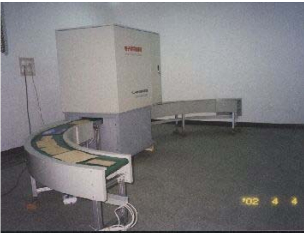
Figure 13: 2MeV electron linac for protecting mail against anthrax.
