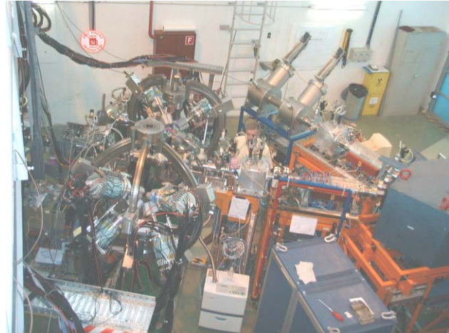
Figure 2: The target area of REX-ISOLDE. The MINIBALL is at the end of the 65^\circ beamline. At the 20^\circ beamline the target chamber for the Li run has been removed and was replaced by an emittance scanner (background right hand side) for commissioning measurements.
