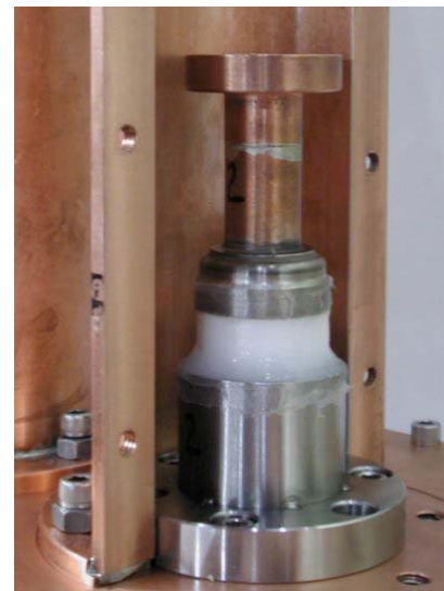
Figure 4: Modified feedthrough with shield
