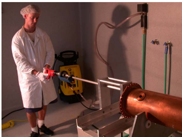
Figure 3: The manual high pressure water rinse system shown with the copper 'dummy' cavity.
