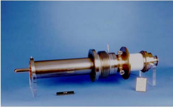
Figure 3: LEP coupler as example of a one window design
