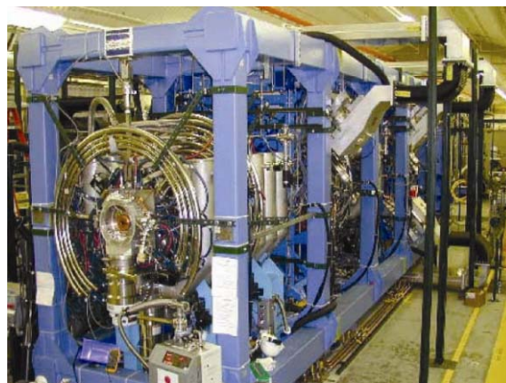
Figure 7: View of the LEDA RFQ after installation
