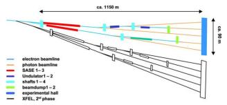
Figure 2: The 1<sup>st</sup> stage user beamline layout (coloured) and the possible extension.
