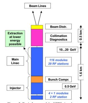
Figure 3: Basic Layout of the XFEL Accelerator.
