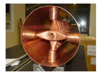
Figure 6: The full scale CH-prototype in copper.
