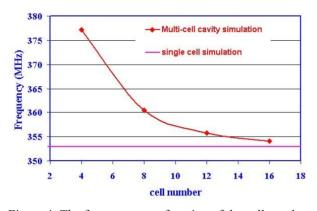
Figure 4: The frequency as a function of the cell numbers.
