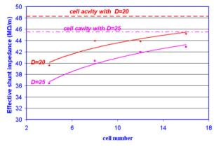
Figure 5: The effective shunt impedance as a function of the cell numbers.
