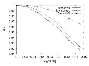
Figure 1: The relative luminosity as a function of a coherent gradient error in the main linac.
