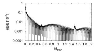
Figure 2: The maximum main beam final energy error due to the drive beam phase jitter resulting from an RF phase error of  $0.01^{\circ}$  in the second drive beam bunch compressor stage as a function of the frequency of the RF error. The results for an RF amplitude error in the same stage of  $2.8 \times 10^{-4}$  are comparable.
