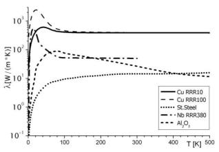
Figure 5b: Thermal Conductivities with Temperature.
