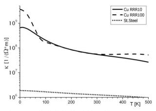
Figure 5a: Electrical Conductivities with Temperature.
