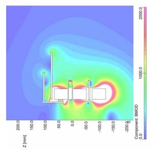
Figure 2: Magnetic simulations with shielding and discs.
