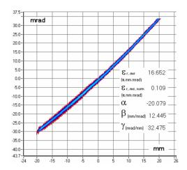
Figure 5: First beam emittance measurement ( $D^+$  current = 4.2 mA).
