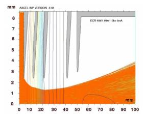
Figure 3: 4.8 mm diameter hole extraction system.
