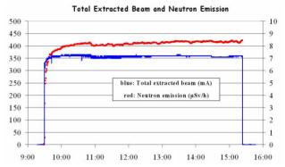
Figure 6: Neutron Emission and Extracted Current vs time.
