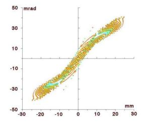
Figure 4: Emittance at 7.6 mm from extraction hole.
