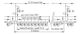
Figure 2 : A simplified scheme of the equipment and instrumentation of a XFEL-linac cryogenic string, which consists of 12 cryomodules, is shown. 'Q' corresponds to a superconducting magnet package.
