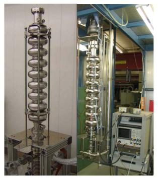
Figure 2: TESLA Cavities for BESSY during HPR at ACCEL (left) and vertical testing at DESY (right).
