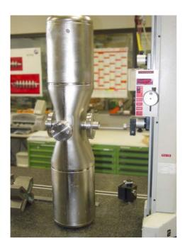
Figure 12: Bulk niobium 176 MHz half wave resonator for the prototype superconducting module for SARAF.
