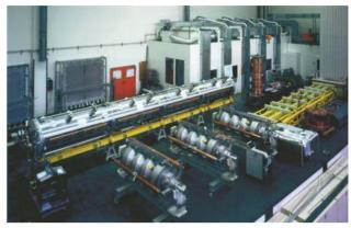
Figure 4: LEP 200 module and 3 single cavity/LHe tank assemblies in our assembly hall. In the back is a 15 m long clean room, the quality of which has since been improved from class 100/10 to class 10/1.
