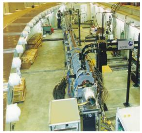
Figure 9: Turn-key S-Band injector linac for SLS at PSI.
