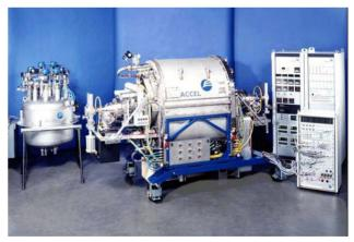
Figure 5: Cornell type module with electronics and valvebox delivered to NSRRC and CLS.
