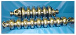
Figure 1: SNS (upper) und TESLA (lower) Cavity.
