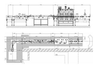
Figure 10: Scheme of the proton/deuteron injector linac for SARAF/Israel.
