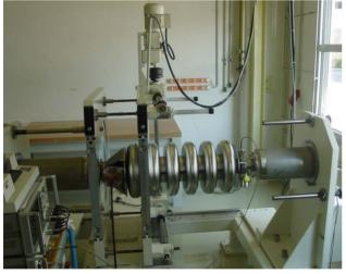
Figure 4: Tuning apparatus for SNS medium beta and high beta cavities. A field flatness of +/-1% in amplitude is easily achieved.
