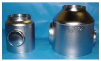
Figure 1: Raw end groups produced for SNS cavities by deep drawing and nipple pulling from one reactor grade niobium sheet.
