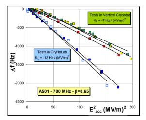
Figure 6: K<sub>L</sub> experimental measurements in vertical cryostat and CryHoLab.
