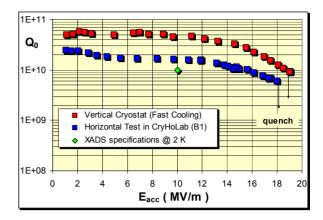
Figure 3: Q<sub>0</sub> vs. E<sub>acc</sub> in vertical and horizontal cryostats.
