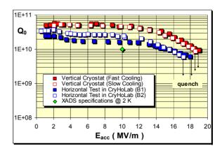
Figure 4: Q<sub>0</sub> vs. E<sub>acc</sub> for A5-01 at 1.7 K showing the influence of magnetic shielding and slow cooling down.
