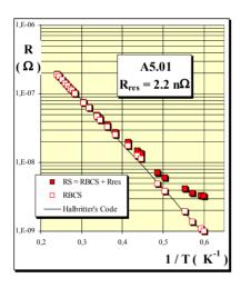
Figure 2: Surface resistance measurement between 4.2 and 1.7 K fitted by the BCS theory.
