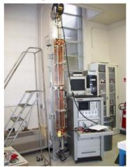
Figure 11: Wire measurement set-up with the RDDS1 structure.
