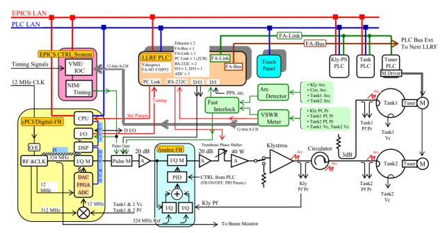
Figure 1: Block diagram of LLRF System.
