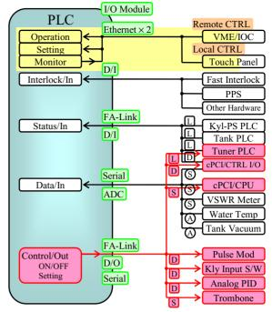
Figure 2: Control flow from/to the PLC.
