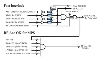
Figure 4: Block diagram of the Fast Interlock module.
