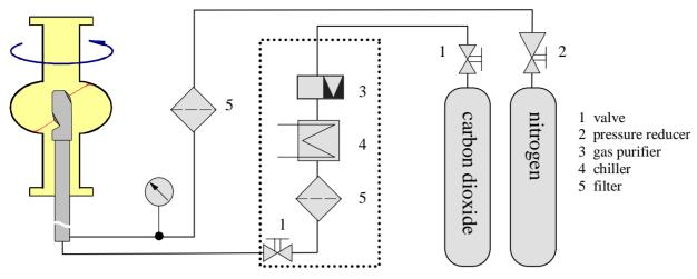
Figure 1: Schematic of the prototype set up for dry-ice cleaning of monocell cavities.
