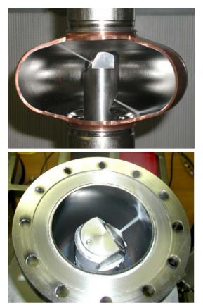
Figure 3: Nozzle test in a cut NbCu cavity (top) and in the beam tube of a Nb monocell (bottom).
