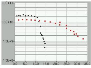
Figure 4:  $Q(E_{acc})$ -performance of a monocell cavity at 2 K before (black) and after (red) dry-ice cleaning.
