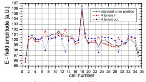
Figure 2: AC- field amplitudes for different tuner positions.
