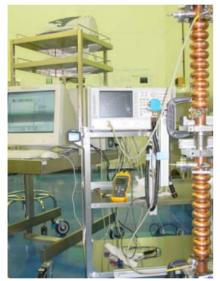
Figure 7: HOM studies of assembly of the two copper cavities on the bead-pull set-up in clean room.
