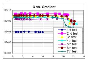
Figure 4: Q-value vs. Accelerating gradient in 3<sup>rd</sup> harmonic 3-cell cavity.
