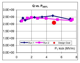
Figure 6: Q-value vs. kick gradient in CKM cavity.
