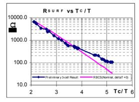
Figure 5: Surface resistance vs. T<sub>c</sub>/T for CKM cavity.
