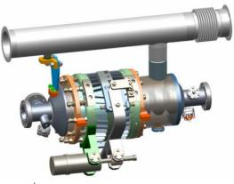
Figure 1: 3<sup>rd</sup> cavity, equipped with helium vessel and frequency tuner (design).
