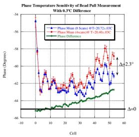
Figure 3: Phase sensitivity as a function of temperature. Error bars represent phase error for number of scans. Temperature standard deviation calculated from a sum of data for all scans in group.
