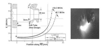
Figure 6: Maximum electric field between the first big drift tube (housing a triplet lense) and the subsequent small drift tube (left); before the improved drift tube geometry was applied (right).
