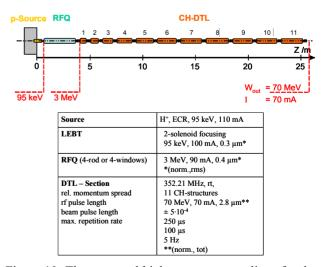
Figure 10: The proposed high current proton linac for the injection into the SIS 18 [5].
