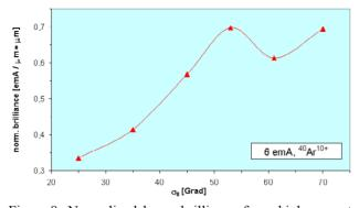
Figure 8: Normalized beam brilliance for a high current argon beam after the 4<sup>th</sup> Alvarez-tank as a function of  $\sigma_0$ .
