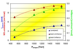
Figure 7: Measured  $U^{28+}$ -current, -emittance and brilliance after charge state separation as a function of the stripper gas density; the input  $U^{28+}$ -current is 6 emA.
