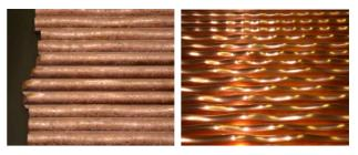
Figure 3: Upgrade of the HSI-RFQ; RFQ-electrodes after five years of operation (left), new electrodes before assembly (right).
