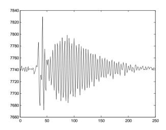
Figure 1: Sample IF waveforms from the ATF/BINP/SLAC cavity BPMs. The vertical scale is ADC counts and the horizontal scale is sample number of the 100 MHz sampling ADC.
