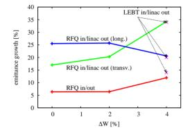
Figure 4: Influence of source energy spread on rms emittance growth.
