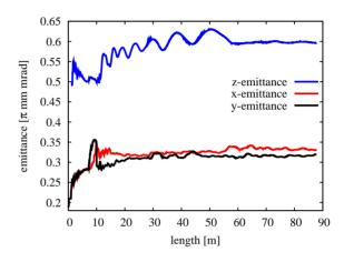
Figure 3: End-to-end (LEBT to 160 MeV) rms emittance evolution (from PATH).
