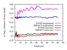
Figure 5: Rms emittance evolution simulated with PATH and IMPACT.
