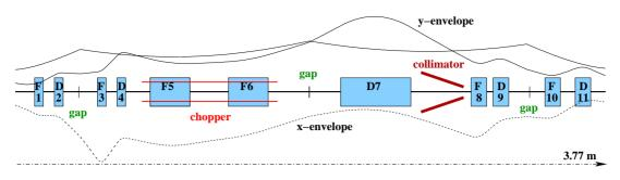
Figure 2: Chopper line and beam envelopes from TRACE3D.
