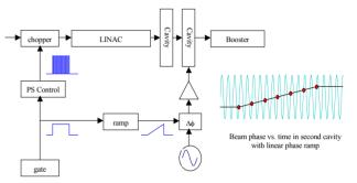
Figure 4: Schematic of the correlated longitudinal painting system. The drive signal to the sweeping cavity is phase modulated with a linearly-increasing phase to sweep the beam across the desired range of phase over the macropulse. The modulation is synchronized with the chopping pattern and the booster RF.
