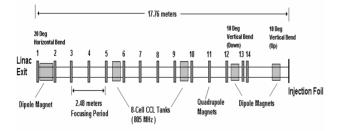
Figure 1: Unfolded layout of the booster transfer line.
