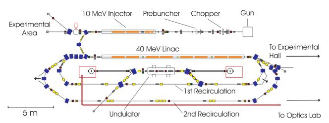
Figure 1: Layout of the S-DALINAC.
