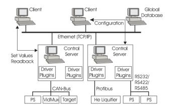
Figure 2: Layout of the control system, where PS denote a power supply for the magnets and VidMux denotes the Video Multiplexer.
