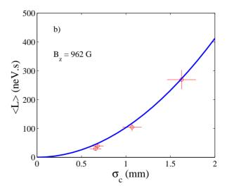
Figure 4: Angular momentum versus charge **a**) and photocathode drive-laser spot size **b**). The experimental data (circles) are compared with theoretical value of the canonical angular momentum calculated from the longitudinal magnetostatic field. In **a**), the dashed line represent the average value of all the data points, and the shaded area corresponds to the uncertainty on the canonical angular momentum.
