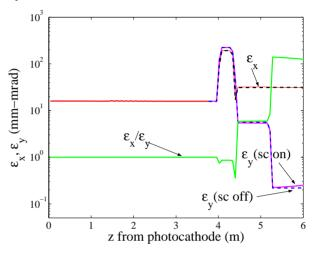
Figure 2: Simulated evolution of transverse emittances along the FNPL beamline for standard nominal settings.
