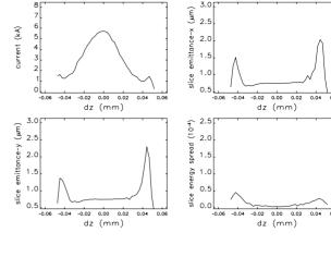
Figure 4: Slice parameters at the end of XFEL linac.
