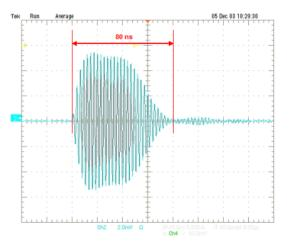
Figure 3: Measured TD impulse response of the band-pass input filter – stripline version of the read-out electronics.
