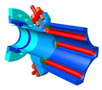
Figure 2: Sectional view of a TTF2 stripline-BPM.
