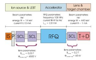
Figure 1: Schematic drawing of the experimental set up.
