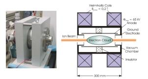
Figure 5: Picture and cross sectional view of the high field Gabor lens.
