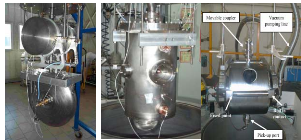
Figure 4: Reentrant cavity and HWR ( \beta=0.31 ) prototypes, developed at LNL, and Spoke cavity ( \beta=0.35 ) prototypes developed at CNRS Orsay.
