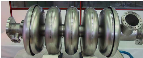
Figure 2: Prototype of a \beta=0.65 , 5-cell cavity fabricated in France.
