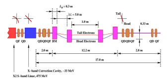
Figure 8: Detail layout of BC1.
