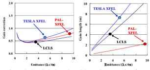
Figure 3: 3D Gain length and 3D gain correction factor.
