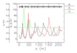
Figure 6: Lattice profile along the linac.
