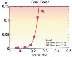
Fig. 8 Peak output power v.s. bunch charge. Using photo diode, peak height was detected from averaged pulses.
