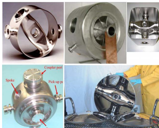
Figure 2: Spoke cavities. Clockwise from top left; ANL 805 MHz \beta=0.28 , IPN-Orsay 352 MHz \beta=0.35 , Jülich 760 MHz \beta=0.2 , ANL 350 MHz \beta=0.63 , LANL 350 MHz \beta=0.17 .
