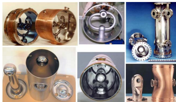
Figure 1: Quarter-wave cavities. Clockwise from top left; ANL 97 MHz \beta=0.07, 0.1 , Stony Brook 150 Mhz \beta=0.06, 0.1 , New Dehli 97 MHz \beta=0.1 , ANL 425 MHz \beta=0.155 , INFN-LNL 160 MHz, ANL 115 MHz \beta=0.15 .
