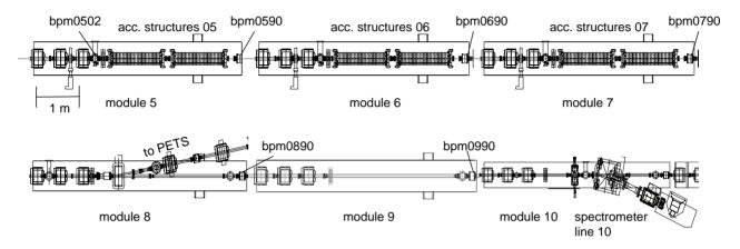
Figure 2: Layout of the CTF3 Linac up to module 10.
