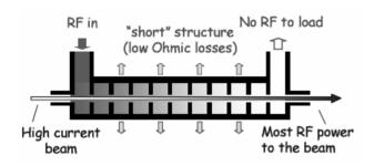
Figure 3: Principle of fully beam-loaded acceleration: A high-current long pulse extracts most of the RF power from a short travelling wave structure.
