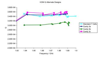
Figure 4: HOM Q for alternate cavity designs.
