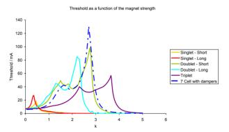
Figure 1: Current threshold vs. k value.
