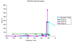
Figure 5: HOM R/Q for alternate cavity designs.
