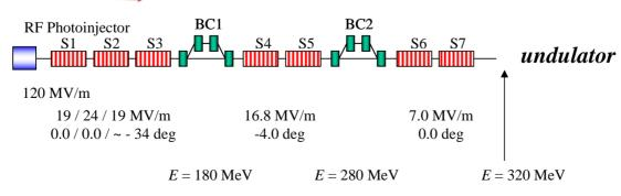
Figure 2: Layout of the test linac.
