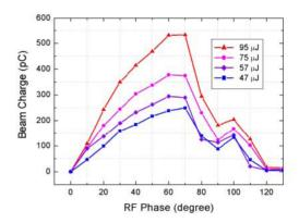
Figure 5: Measured beam charge under various RF phases and laser energies.
