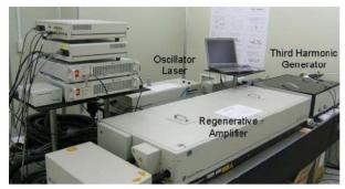
Figure 3: A picture of Ti:sapphire system.
