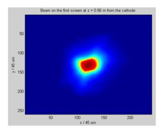
Figure 4: Electron beam image from the GTS gun on a phosphor screen.
