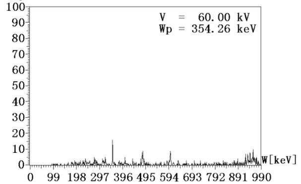
Figure 6: Simulated energy spectrum at 60kV ( $O^+$  beam, input energy 22.4keV, 26MHz).
