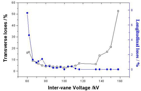
Figure 5: Particle loses vs inter-vane voltage ( $O^+$ , input energy 22.4keV,  $f=26\text{MHz}$ ).
