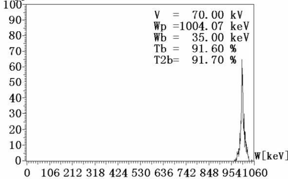
Figure 9: Simulated energy spectrum at 70kV ( $O^+$  beam, input energy 22.4keV, 26MHz).
