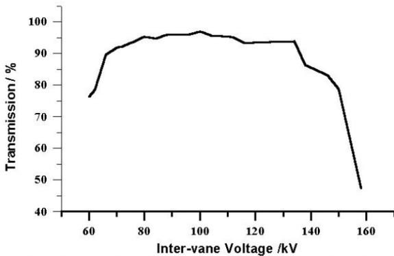
Figure 5: Beam transmission vs inter-vane voltage ( $O^+$ , input energy 22.4keV,  $f=26\text{MHz}$ ).
