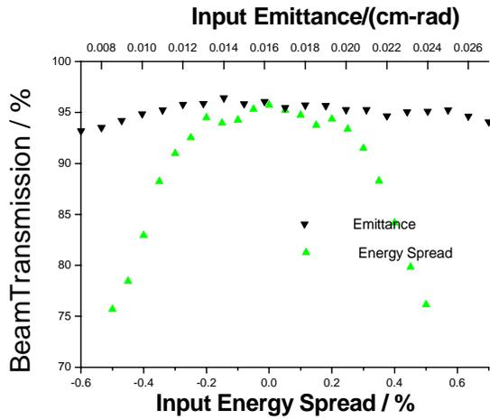
Figure 4: Beam transmission vs different input emittance and energy spread.
