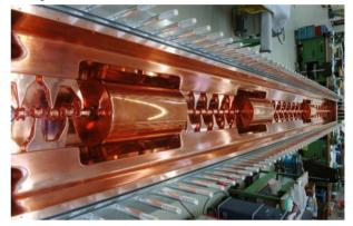
Figure 8: Open IH cavity after copper plating and assembly of the drift tubes. Each of the three large drift tubes contains a magnetic quadrupole triplet lens.
