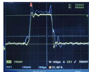
Figure 9: Beam current signals from the ACCTs.
